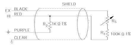
FIGURE 7-2. 237 Sensor Schematic
