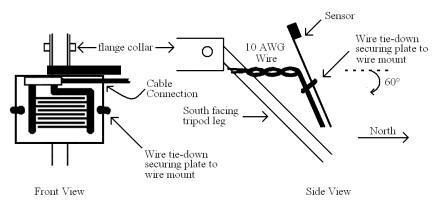
FIGURE 7-1. Example 237 Field Installation
